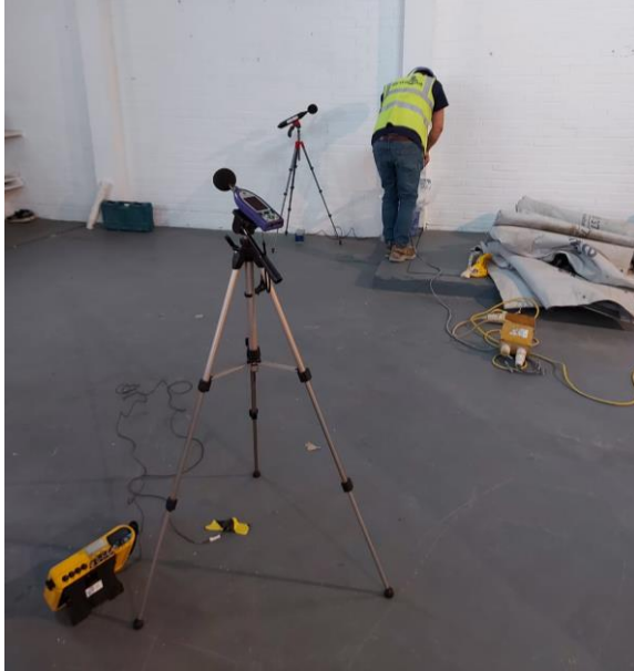
A3.1: Test No. 1 – Boring Holes to Coring Column, Lobby, Ground Floor.
