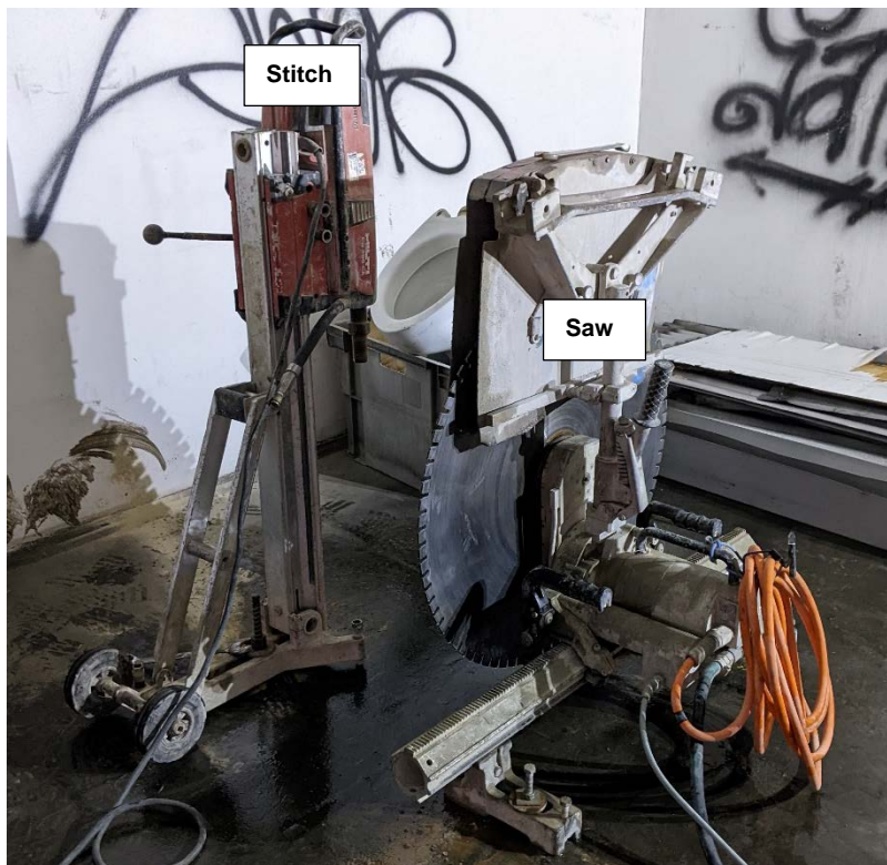
A4.3: Stitch (core) Drill and Floor Saw
